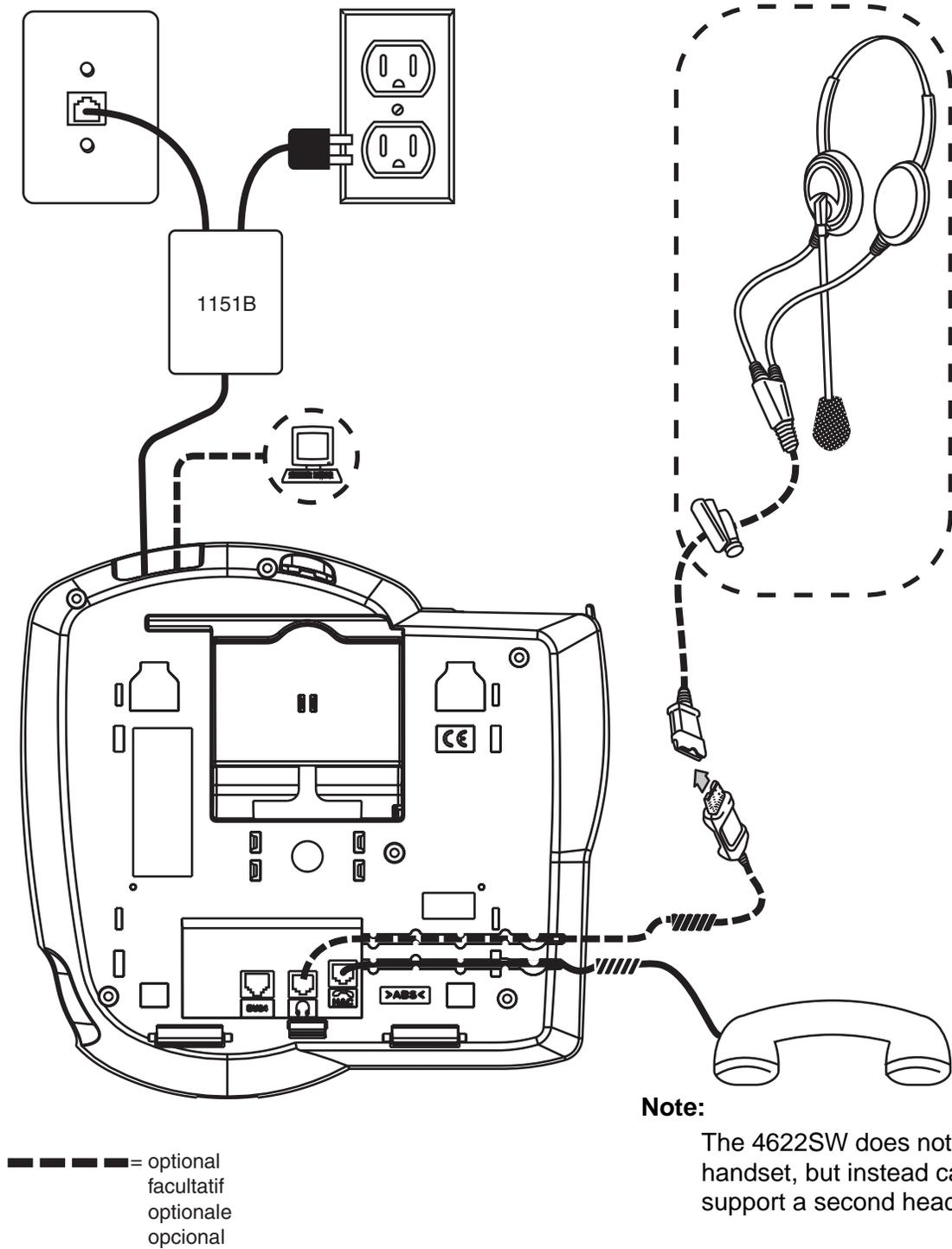
Figure 5: Connection Jacks on a 4610/4620/4620SW/4621SW/4622SW/4625SW/4630SW IP Telephone - Option B
