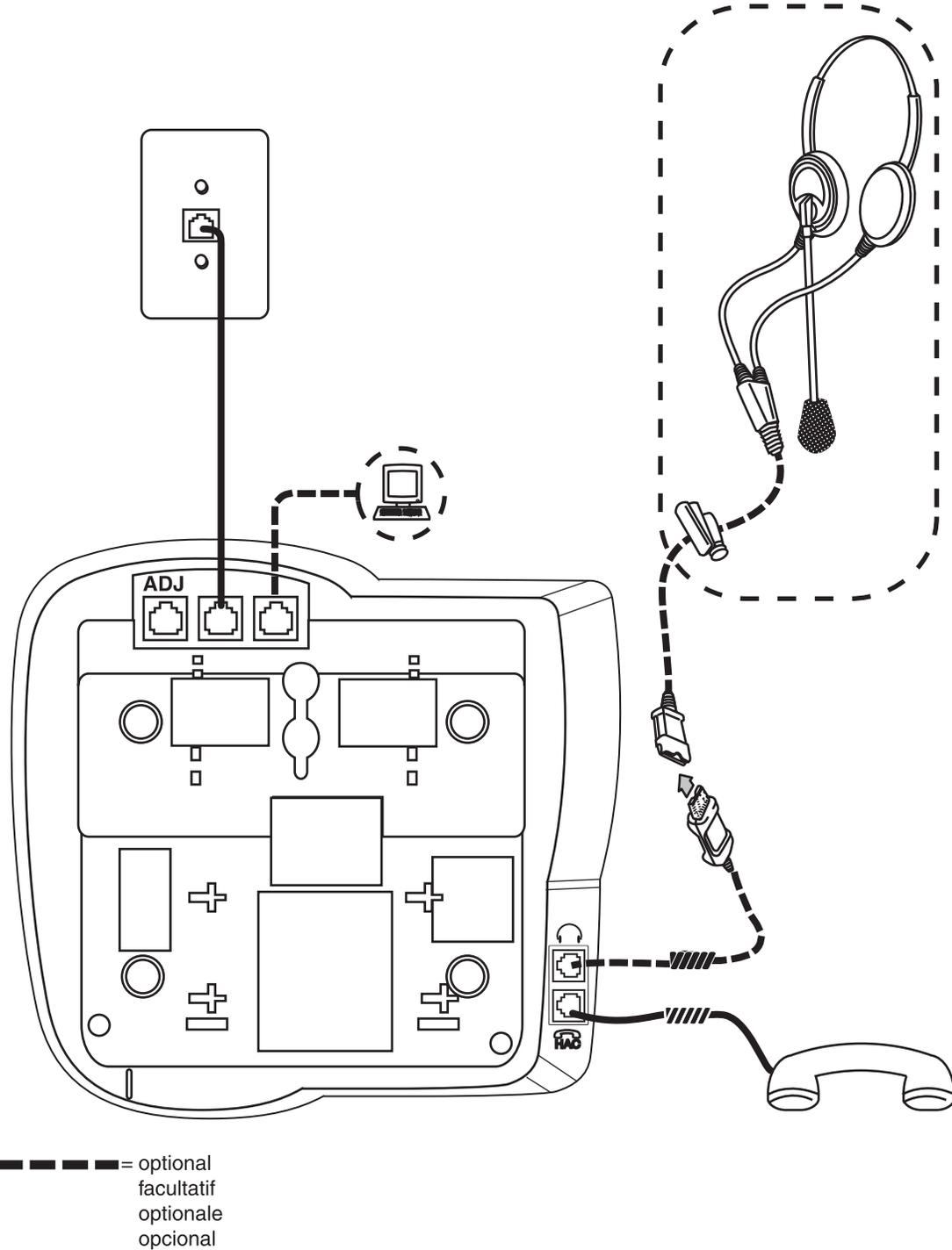
Figure 11: Connection Jacks on a 4690 IP Conference Telephone
