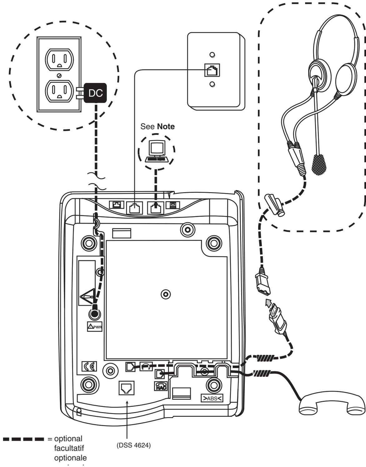
1. Plug one end of the H4DU 4-conductor coiled handset cord into the telephone and the other end into the handset.
