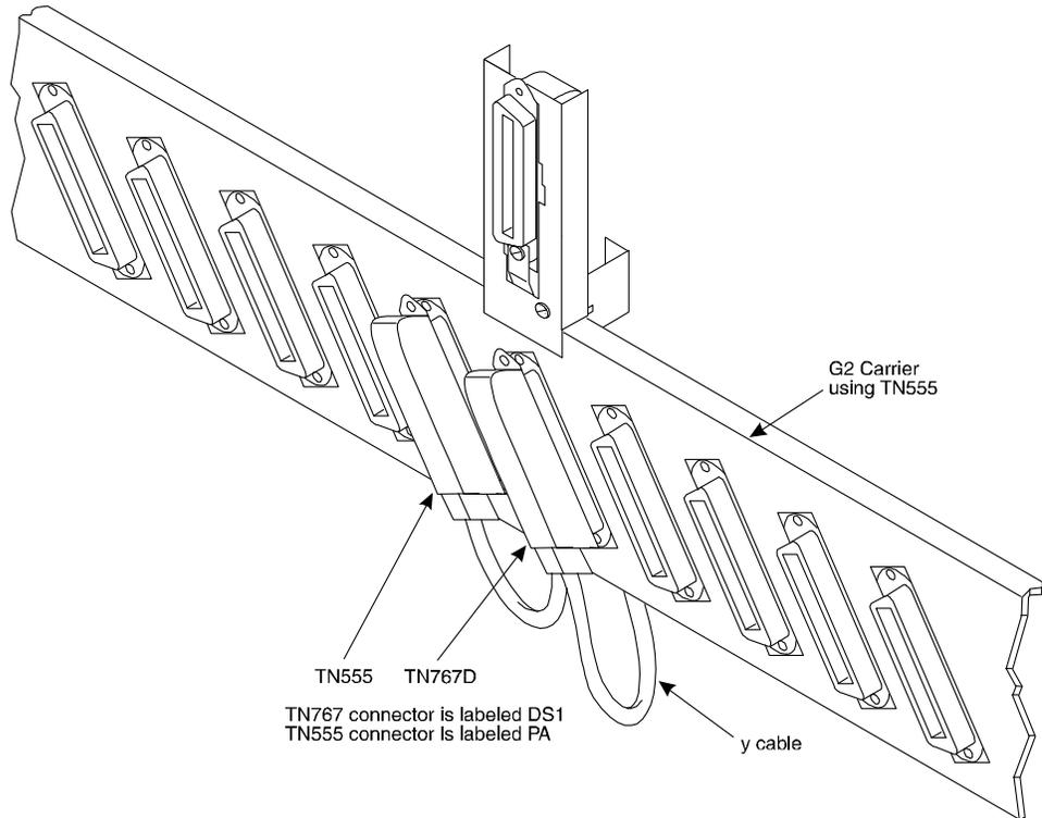
4. Attach the CSU module with a 4C retainer to the 50-pin connector on the connector bracket as described in the following section.
