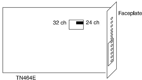
9. Set the line compensation value for 0-133 feet. This is the distance between the DS1 circuit pack and the CSU module. This is set from the switch administration terminal. In G1 and G3 systems you do this in the DS1 circuit pack form in the field **line compensation**. In G2 systems, you do this in procedure 260, word 1, field 18. This setting should not be confused with the distance from the CSU module to the smart jack which is automatically compensated for by the CSU module.
