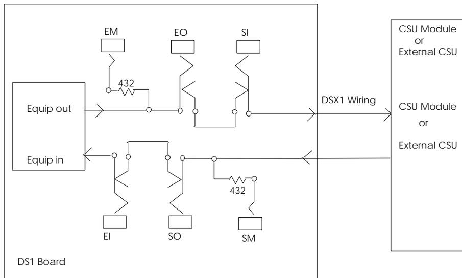
**Figure 6. Test Jacks Circuitry**
