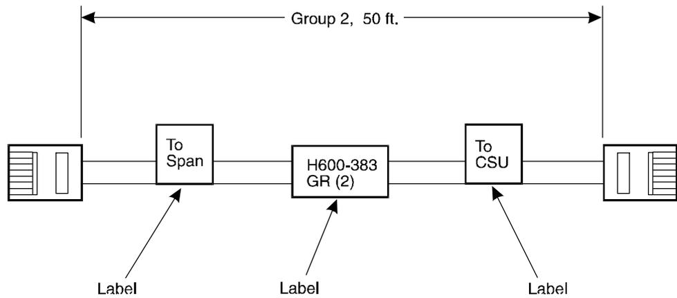
**Figure 3. H600-383 CSU-to-Network Smart Jack Cable**
