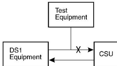
**⇒ NOTE:** Inserting test equipment into only this jack kills the signal to the CSU module. This causes the integrated CSU module to raise an alarm indicating loss of signal from the DS1 circuit pack. This in turn causes the CSU module to loop the span back to itself. Thus, to avoid this alarm, you should use the EM jack instead or also provide a signal to the CSU module via the SM In jack.
