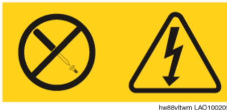
Hazardous voltage, current, and energy levels are present inside any component that has this label attached. There are no serviceable parts inside these components. If you suspect a problem with one of these parts, replace the power supply.
