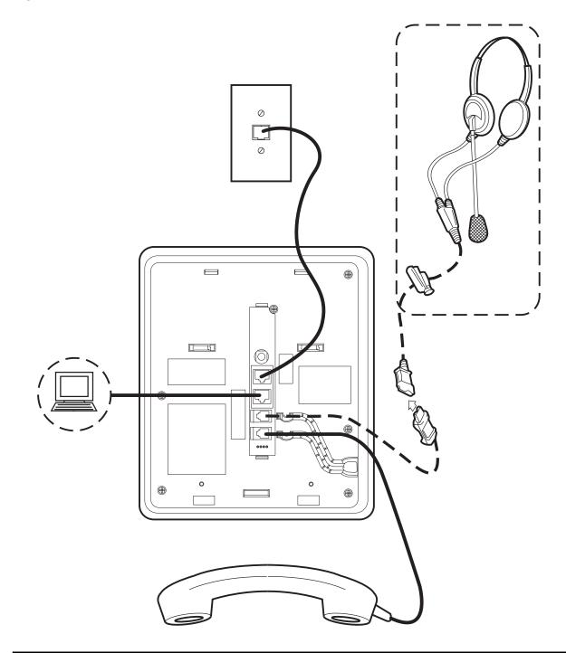
Figure 4: Connection Jacks with Power over Ethernet on a 1608/1608-I IP Telephone
