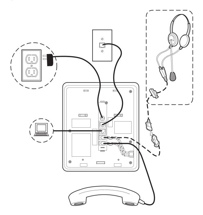
Figure 5: Connection Jacks with Local Power on a 1608/1608-I IP Telephone
