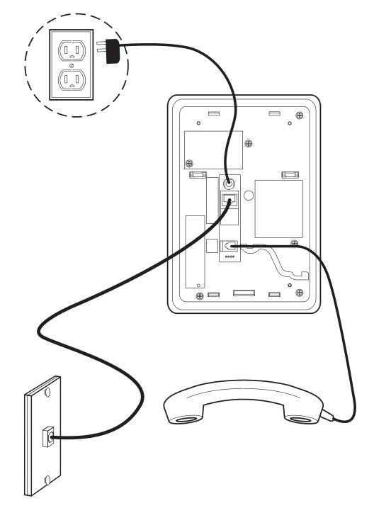
Figure 2: Connection Jacks with Local Power on a 1603/1603-I IP Telephone
