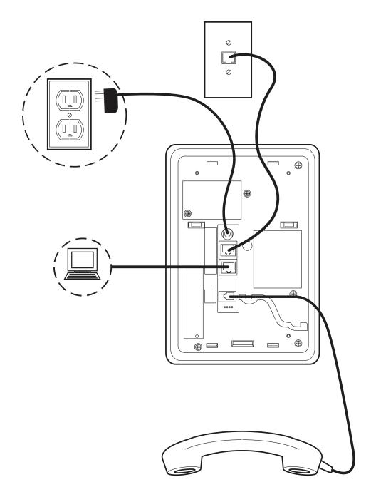
Figure 3: Connection Jacks on a 1603SW/1603SW-I IP Telephone
