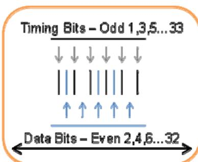
The LCW (16 Even Data Bits) has the following structure and definitions:
