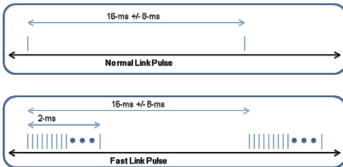
Of the 33 FLP pulses, there are 17 odd pulses used for timing and 16 even pulses used for data settings. The 16 data pulses are called the Link Code Word (LCW). The diagram below shows the timing and data pulses. Timing bits are always present. Data bits are only present to indicate a value of one and are absent to indicate a value of zero.
