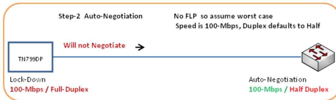
One can see that when one side of a link has speed/duplex locked down, the other side using Auto-Negotiation will always set itself to the correct speed, but uses half-duplex because it assumes the lock-down device is a very old NIC that uses half-duplex.
