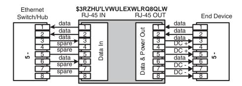
For Data-In ports connect the Ethernet cable leading from the Ethernet Switch/Hub to the Data port. For Data & Power Out ports, connect the Ethernet cable leading to the telephone or other end device to the corresponding Data & Power port.
