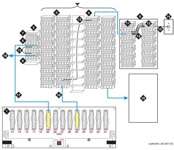
Figure 2: Example MDF connections (G650 Media Gateway)
