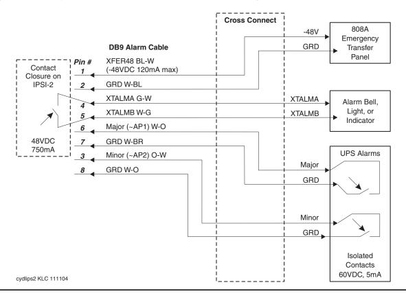
Figure 41: Sample Issue 1 IPSI-2 alarm cable connectivity
