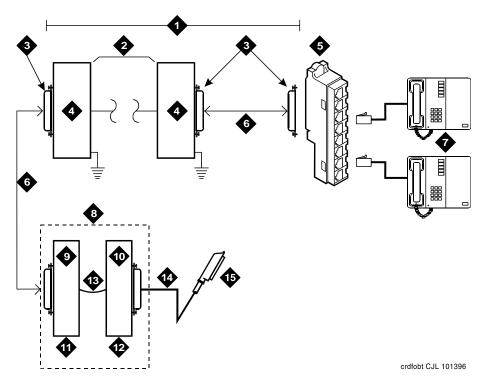
Figure 42: Connections for 1 to 8 out-of-building analog telephones
