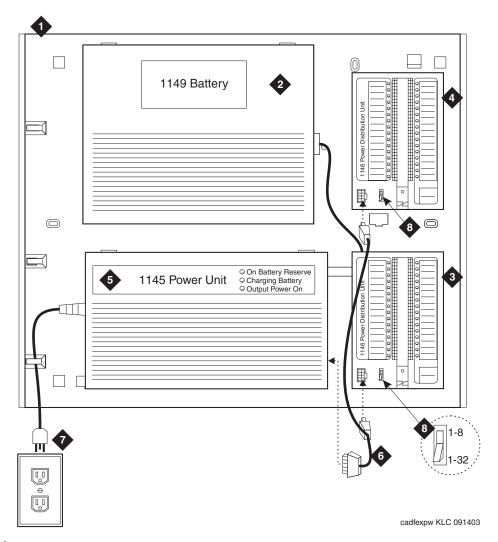
Figure 51: Expanded power distribution unit
