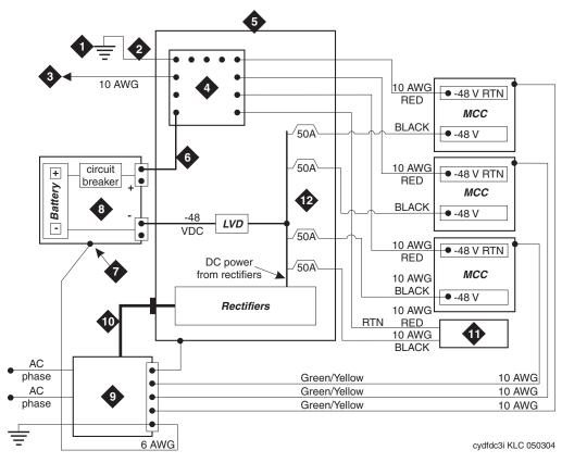
Figure 25: Typical power and ground for a DC power cabinet
