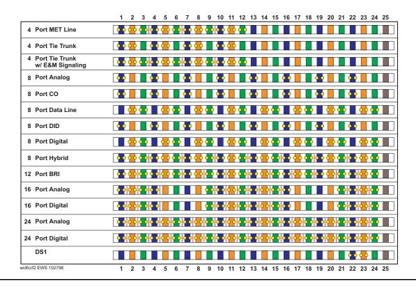
Figure 2: Example MDF connections (G650 Media Gateway) on page 25 shows a detailed example of the G600 Media Gateway cables connecting media gateways and satellite closets to the MDF. This figure shows the cross-connections for one example station circuit.
