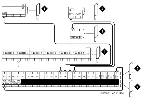
Figure 48: Connections for telephone used for emergency transfer and as normal extension
