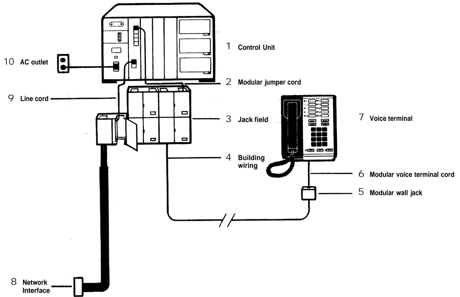
You must also have a network interface that links your system to the local telephone company's lines. A telephone company representative should have installed the necessary outside telephone lines and labeled the network interface to indicate the telephone number for each outside line. Depending on the type of interface provided by the telephone company, your system may require additional wiring running from the network interface to the jack field.
