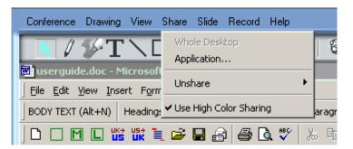
The color depth is 8 bits per pixel (256 colors) for High Speed sharing, or 24 bits per pixel for High Color sharing.
