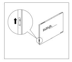
To insert the PC Card, hold it with the label facing to the right, and slide it gently into one of the PC Card slots on the processor module. When inserted properly, the PC Card projects about 1-5/8" (4 cm) from the module.
