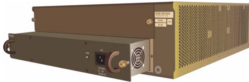
Figure 31: Replacing a power supply unit
