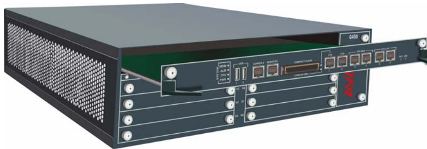
Figure 25: Removing and inserting the G450 main board
