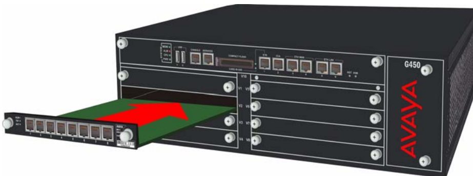
Figure 8: Inserting a media module
