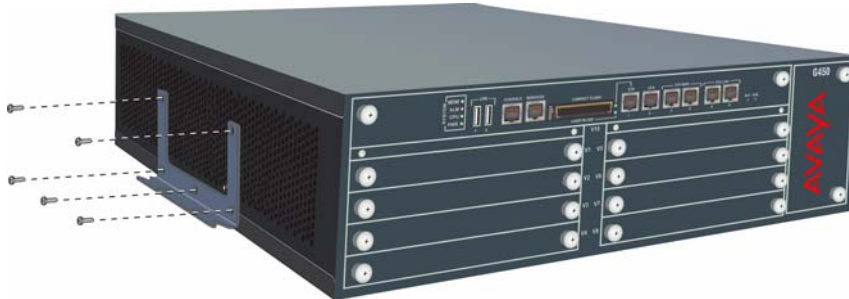
Figure 4: Attaching a bracket to each side of the G450
