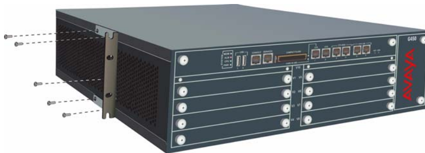
Figure 2: Attaching a mounting bracket to the middle of the G450
