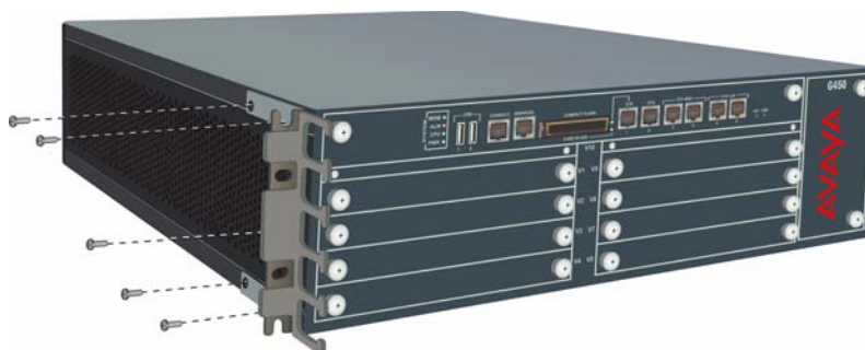
Figure 3: Attaching a mounting bracket with cable guides
