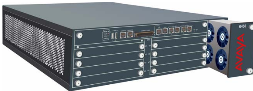
Figure 30: Replacing the fan tray
