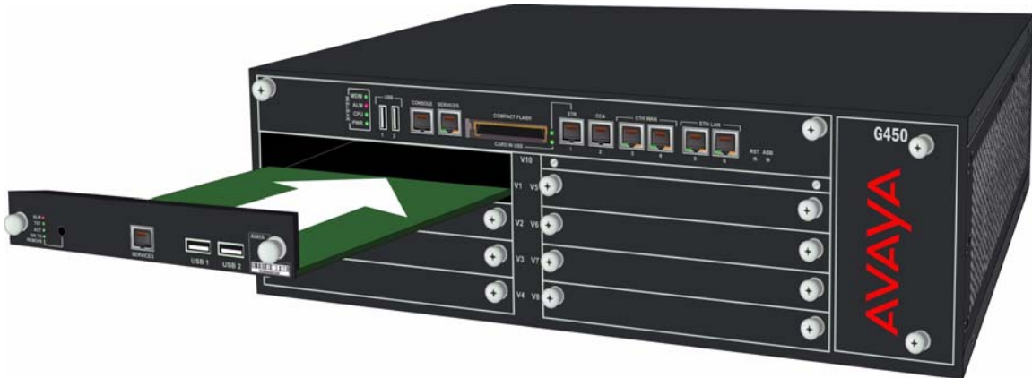
Figure 7: Inserting the S8300 Server
