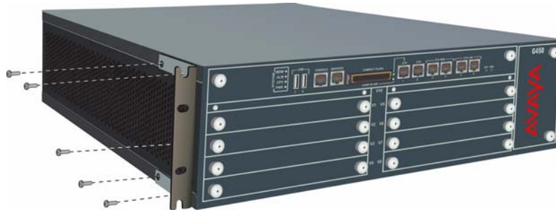
Figure 1: Attaching a mounting bracket to the front of the G450
