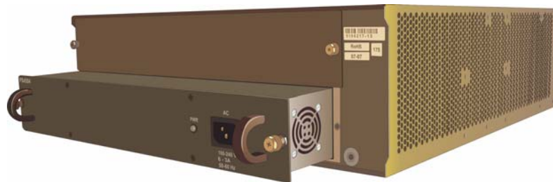
Figure 5: Inserting the power supply unit
