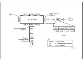
In "802.1Q tag assignment" (page 206), tagged incoming packets are assigned directly to VLAN 2 because of the tag assignment in the packet. Port 5 is configured as a tagged member of VLAN 2, and port 7 is configured as an untagged member of VLAN 2.
