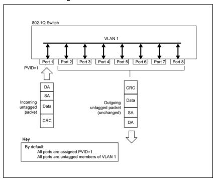
When you configure VLANs, you configure the switch ports as tagged or untagged members of specific VLANs (see "Port-based VLAN assignment" (page 205) through "802.1Q tagging - after 802.1Q tag assignment" (page 206)).
