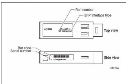
SFPs are hot-swappable products that enhance input and output and allow gigabit Ethernet ports to link with other gigabit Ethernet ports over various media types. "1000BASE-SFP models" (page 200) lists and describes the Nortel SFP models that are supported by the BES100 and BES200 Series switches.
