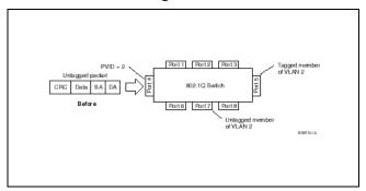
As shown in "802.1Q tagging (after port-based VLAN assignment)" (page 205), the untagged packet is marked (tagged) as it leaves the switch through port 5, which is configured as a tagged member of VLAN 2. The untagged packet remains unchanged as it leaves the switch through port 7, which is configured as an untagged member of VLAN 2.
