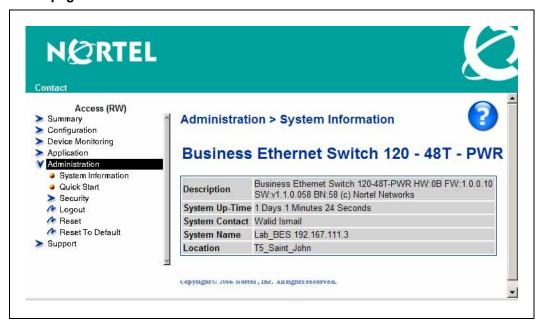
The figure shows the home page for the BES120-48T PWR 48-port switch. Other than the number of fixed ports, there are no major differences between the 24-port and 48-port switch user interface. The home page for the BES200 Series switch shows content similar to what is shown in this figure, however the content is specific to the BES200 series switch.
