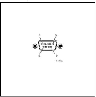
"DB-9 console port connector pin assignments" (page 234) lists the DB-9 console port connector pin assignments.
