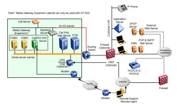
In the illustration "Sample network setup: Communication Server 1000" (page 17), the telephony LAN (TLAN) provides IP connectivity between the Communication Server 1000 Expansion switch and the i2004 Internet telephones. The connection between the Call Server and Media Gateway Expansion can be point-to-point, or it can be through the LAN, if the system is installed in a distributed data network.
