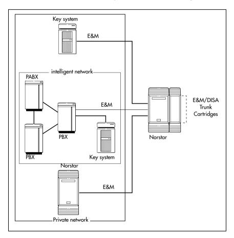
By default, auto-answer E&M trunks are answered by the system with direct inward system access (DISA), and are used to provide controlled access to Norstar system resources.
