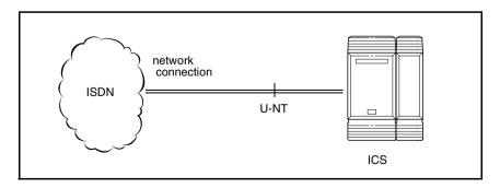
U-NT and U-LT loops can be used in combination to provide D-packet service for a point-of-sale terminal adapter (POSTA) or other D-packet device. D-packet service is a 16 kbps data transmission service that uses the D-channel of an ISDN line.
