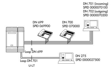
The following table uses the example in the illustration to show the programming for the S loop.
