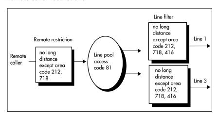
In this case, dialed digits must pass both the remote restriction and the line restriction. A remote caller can override these filters by dialing the DISA DN and entering a COS password.
