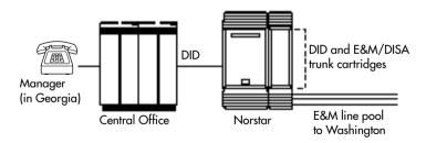
**Hardware:** ICS, a Trunk Module with a DID Trunk Cartridge, two E&M/DISA Trunk Cartridges for the three trunks in the line pool to Washington, or a DTI with one DID line and three E&M lines.
