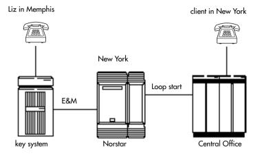
**Hardware:** ICS, a Trunk Module with an E&M/DISA Trunk Cartridge or DTI with an E&M line.
