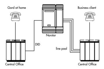
**Hardware:** ICS, a Trunk Module with a DID Trunk Cartridge or DTI with several DID lines.
