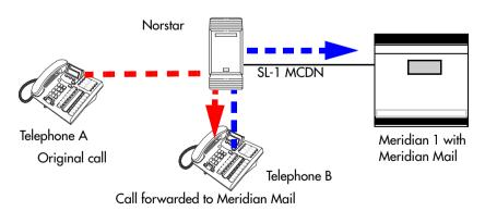
If you are using the centralized voice message system from a Meridian 1 system, you require the following programming on the M1:
