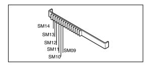
• **Fiber Cable Guide (three per system):** install in the entrance and exit of the cable trough. The Fiber Cable Guide allows fibers to be correctly routed to maintain a minimum bend radius when going through the cable trough.
