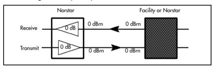
The value High induces 7 dB of loss in the receive path and 16 dB of loss in the transmit path. Use it when the E&M trunks are connected to facilities that present +7 dBm in the receive path and -16 dBm in the transmit path at the interface.
