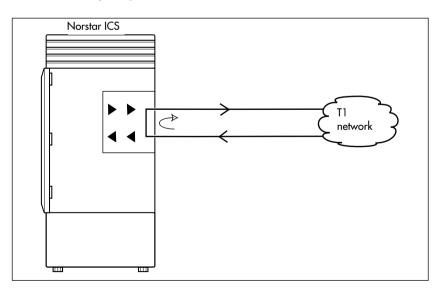
The continuity loopback test shorts the tip and ring pair of the receive signal path with the transmit signal path. This test allows you to check the metallic continuity of the external wiring.
