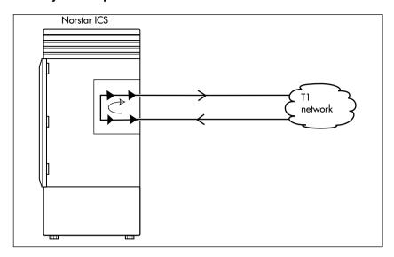
The payload loopback test loops the received information bits (192 per frame) back to the network. The payload loopback test can also be invoked and stopped remotely via the facility data link (FDL) in extended super frame (ESF) format.
