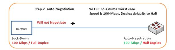
One can see that when one side of a link has speed/duplex locked down, the other side using Auto-Negotiation will always set itself to the correct speed, but uses half-duplex because its assumes the lock-down device is a very old NIC that uses half-duplex.
