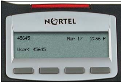
Figure 9: Logged on to an IP Audio Conference Phone 2033 using an IP Phone 2002
