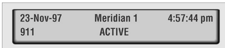
Figure 26: Attendant display when the attendant places an Autoline call to an external Autoline DN
