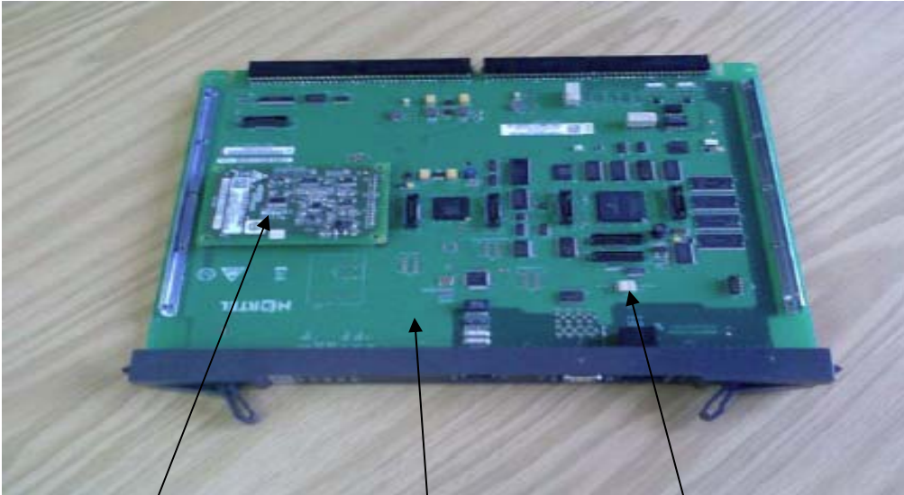
Clock Controller d'board T1/E1 Trunk card DIP switch
