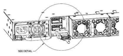
Figure 21: Installing Fabric Interconnect cables
