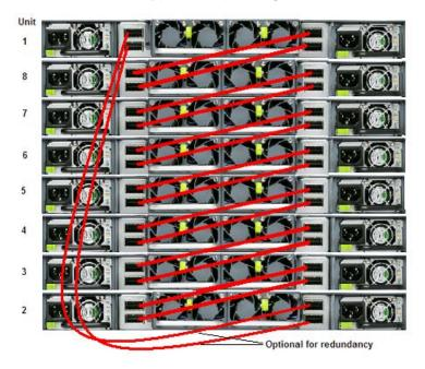
Figure 20: FI up cable configuration
