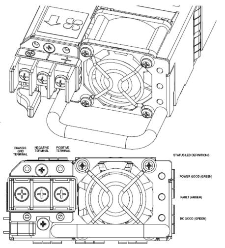
Figure 6: DC power supply terminals
