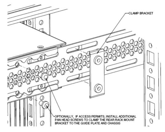
Figure 15: Optional rear bracket screws
