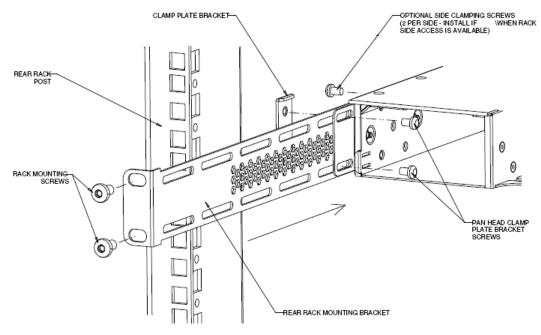
Figure 14: Attach rear mounting brackets
