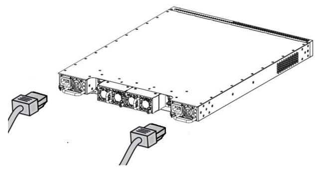
Figure 5: Connecting AC power cord to the switch
