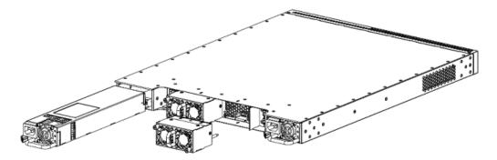
Figure 4: Installing the fan trays and power supplies
