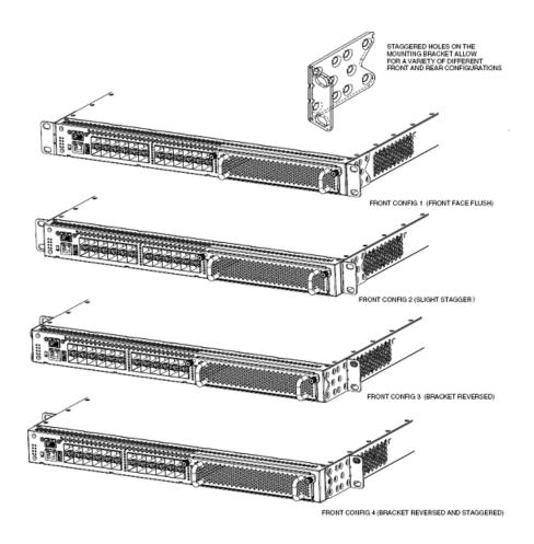
Figure 7: Front-mounted rack bracket installation options
