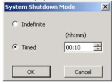
Select the type of shutdown required. If **Indefinite** is used, the system can only be restarted by having its power switched off and then on again. If a **Timed** shutdown is selected, the IP Office will reboot after the set time has elapsed.
