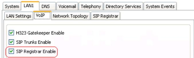
The screenshot shows the IP Office Manager configuration window with the 'System' tab selected. Under the 'LAN1' sub-tab, the 'VoIP' sub-tab is active. The 'SIP Registrar' sub-tab is selected, and the 'SIP Registrar Enable' checkbox is checked and highlighted with a red box. Other checked options include 'H323 Gatekeeper Enable' and 'SIP Trunks Enable'.
