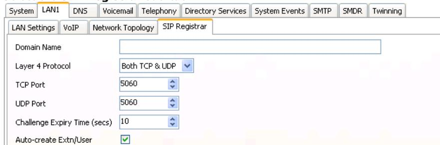
The screenshot shows the IP Office Manager configuration window with the 'System' tab selected. Under the 'LAN1' sub-tab, the 'VoIP' sub-tab is active. The 'SIP Registrar' sub-tab is selected. The configuration fields are: Domain Name (blank), Layer 4 Protocol (Both TCP & UDP), TCP Port (5060), UDP Port (5060), Challenge Expiry Time (secs) (10), and Auto-create Extn/User (checked).
