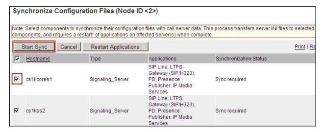
The Synchronization Status field will update from Sync required to Synchronized. After synchronization completes, enter  $\[ \]$  associated with the appropriate Signaling Server and click **Restart Applications** to use the new SIP gateway settings.
