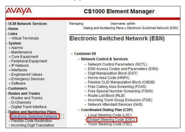
Select **Add** from the drop-down menu and enter the dialed prefix for CS1000E calls to be routed over SIP trunk to Session Manager in the **Please enter a distant steering code** field. For the sample configuration, **44** will be used since SIP endpoints registered to Session Manager were assigned extensions starting with **44**. Click **to Add** as shown below.
