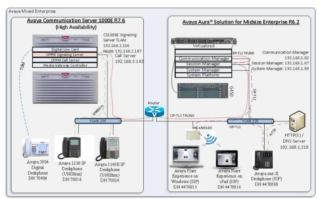
Figure 1 – Network Topology: SIP TLS Trunk between Avaya Communication Server 1000E R7.6 and Avaya Aura® Communication Manager R6.2
