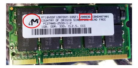
Micron memory modules with later date codes do not need to be replaced. Note that Avaya also shipped memory modules from another supplier (Avant) which do not have the defect and do not need to be replaced.
