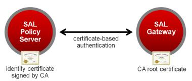
This process is analogous to a web browser authenticating a secure website. The secure web server presents an identity certificate signed by a CA – such as Symantec, for example. The web browser authenticates that identity certificate by using a Symantec root certificate. This certificate-based authentication employs data encryption using a Secure Hash Algorithm (SHA).
