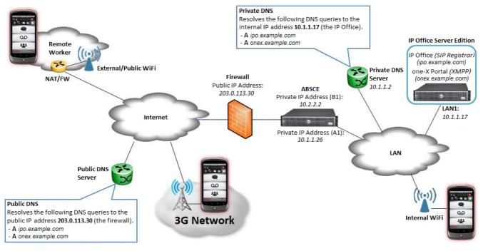
The IP Office is the SIP registrar for telephony services. The one-X Portal for IP Office service connects to the IP Office and in this scenario acts as the XMPP presence provider for the users.
