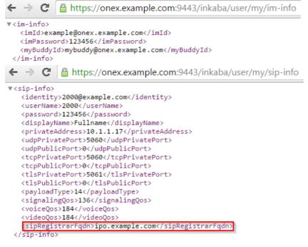
4. The client sends a DNS A query for the IP address of the *sipRegistrarFQDN* received above (the IP Office).
