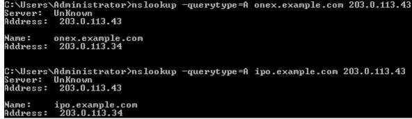
10. Repeat above configuration on the internal DNS server using the private IP of IP Office.
