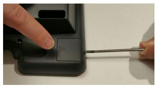
2. To remove the module panel, slide the panel out in the direction of the arrow.
