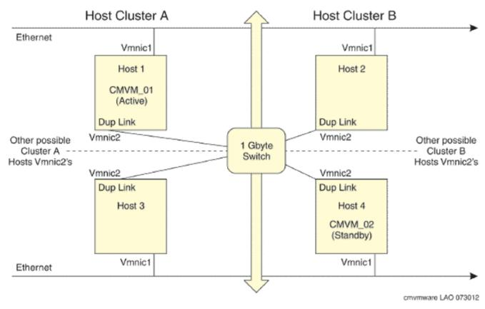
Figure 1: VMware cluster configuration with four ESXi hosts
