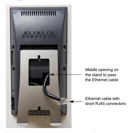
If you use a short cable as suggested, you can fold the extra length of the cable in the space between the stand and the unit.
