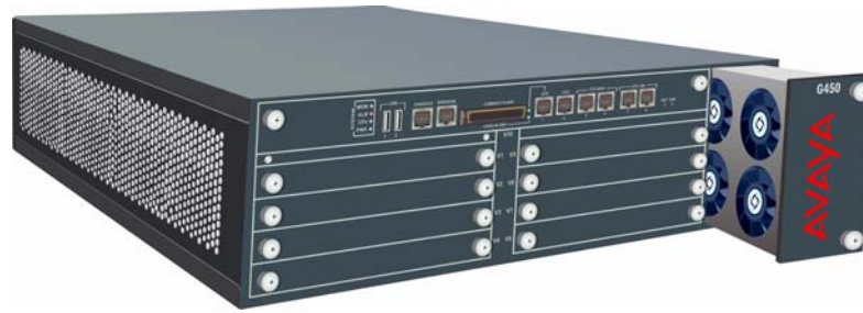
Figure 4: Replacing the fan tray
