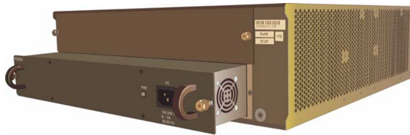
Figure 5: Replacing a power supply unit
