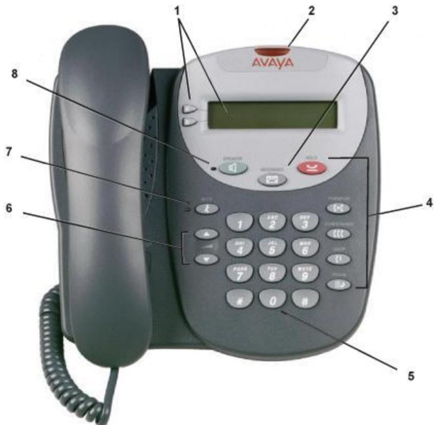
1. **Display and Call Appearance Keys:** Two Call Appearance Keys allow you to handle multiple calls and the display shows call information. Details on system features (allocated by your system administrator) can also be displayed.
