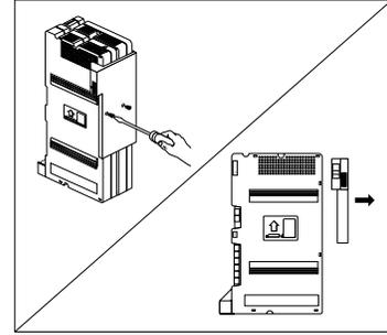
**1** Remove the clear, plastic protector from the connector on the rear of the new module (and the processor module if you are upgrading from a stand-alone system) by grasping the tabs and lifting.
